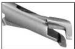
786-1300 Micro distal end cutters T.C with safety hold ● Max. 0.30 mm to 0.50 mm (.012" to .020") ■ Max. 0.46 mm to 0.64 mm (.018" to .025") ⊗ Max. 0.38 mm to 0.53 mm (.0155" to .0215") ⊗ Max. 0.53 mm to 0.64 mm (.021" to .025")
