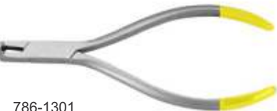
786-1301 Mini distal end cutters T.C with safety hold ● Max. 0.30 mm to 0.50 mm (.012" to .020") ■ Max. 0.46 mm to 0.64 mm (.018" to .025") ⊗ Max. 0.38 mm to 0.53 mm (.0155" to .0215") ⊗ Max. 0.53 mm to 0.64 mm (.021" to .025")
